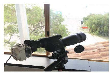
**Figure 35:** GoPro Hero4 Camera attached via lens adaptors to a Redfield 'Rampage' 20-60x60mm Spotting Scope. The CamDo Time Lapse Intervalometer can been seen 'piggy backed' onto the camera which was programmed to take three pictures, one minute apart.
