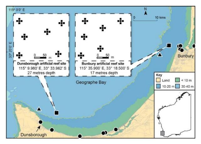
**Figure 39**: Map showing the location of the Bunbury and Dunsborough artificial reefs in Geographe Bay and the configuration of their 30 concrete FishBox modules into six clusters. Grey square on inset denotes the location of Geographe Bay in WA.  $\blacksquare$ , purpose-built concrete reef;  $\blacktriangle$  sunken ship artificial reef; ●, boat ramp. Map modified from the Department of Primary Industries and Regional Development.
