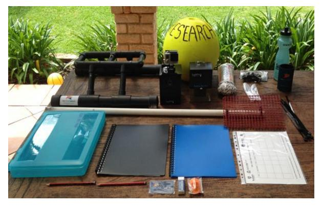
**Figure 41:** The package supplied to volunteers at the workshop including the BRUV unit, promotional material, data storage devices and metadata collection materials.
