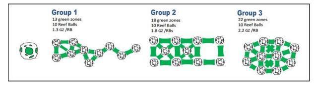
Figure 62: An example of interstitial spaces as 'Green zones' using Reef Ball<sup>TM</sup> modules (Lennon, 2011).
