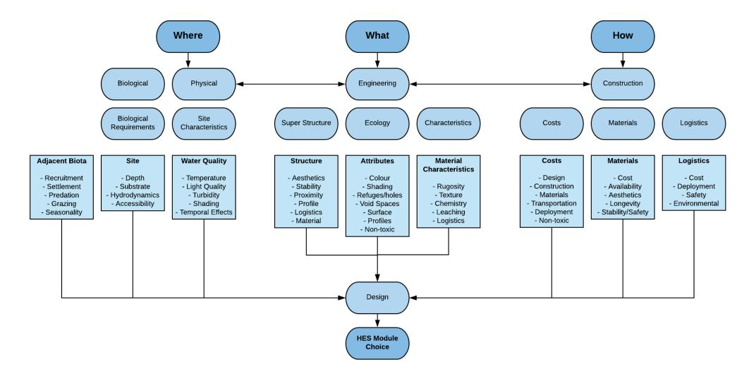
Figure 20: Diagram illustrating the factors influencing HES design. A combination of biological and physical characteristics of the site and target species along with engineering and socio-economic concerns will determine the siting, size and type of HES deployed.
