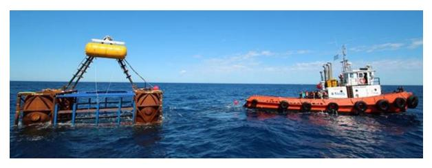
Figure 67: Tug boat towing a 'Fish Tower<sup>TM</sup>' module to its final deployment site.
