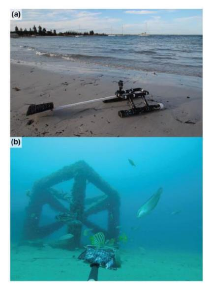
**Figure 42:** Photographs of (a) the BRUVs supplied to Reef Vision participants and (b) a screenshot of footage collected from the Dunsborough Artificial Reef using the BRUV in (a). Footage in b shows 10 *Coris auricularis*, 10 *Neatypus obliquus*, 2 Pseudocaranx spp., 1 *Pentaceropsis recurvirostris*, 1 *Glaucosoma hebraicum* and 1 *Myliobatis australis*.
