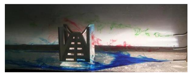
Figure 61: Artificial reef module being tested in a university flume tank (Subcon Pty Ltd).
